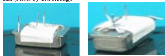
Fig. 11 Above picture shows by bending the QXO leads, it can be fitted in an EXO-3 socket (Photo by CM Heong)
