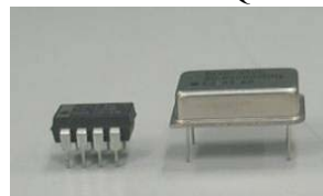
Fig. 10 Picture on the left: EXO-3C. Right: QXO. Note the disparities in size (Photo by CM Heong).
