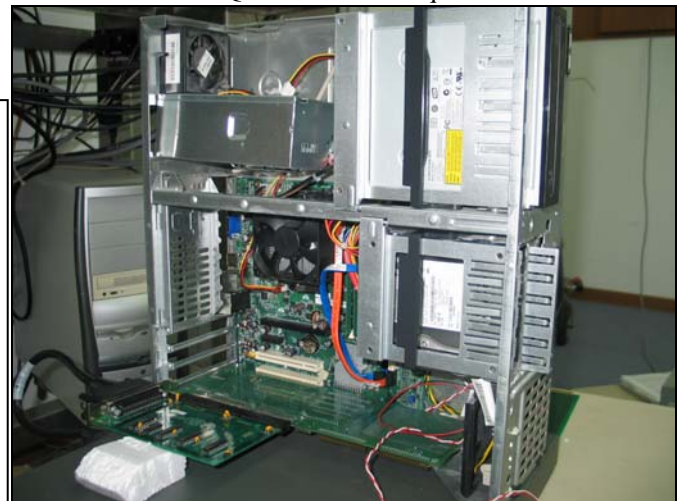
Fig. 9 Photo of desktop with adapter card, with the ISA-bus interface card piggy-backed. Note interface card cable on the bottom left corner. Photo by Emelia Khamis.
